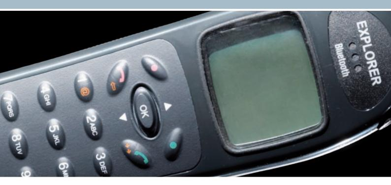
The EXPLORER Bluetooth handset is a cordless telephone handset designed to connect wirelessly via Bluetooth to satellite terminals such as the Thrane & Thrane EXPLORERs. That way you can talk on the phone with anybody anywhere in the world — without strings.
