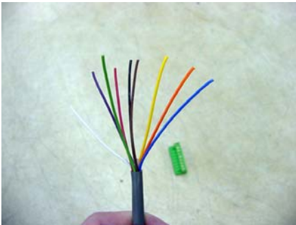
Cut the control cable to length once it has been pulled inside the vehicle. Remove 2" of the plastic cover to expose the wires.
