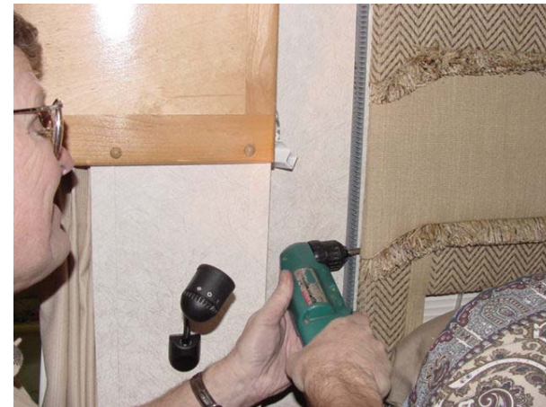
Secure the cable with cable clamps inside the vehicle in inconspicuous areas.
