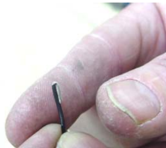
Cut the control cable to length once it has been pulled inside the vehicle. Remove 2" of the plastic cover to expose the wires.
