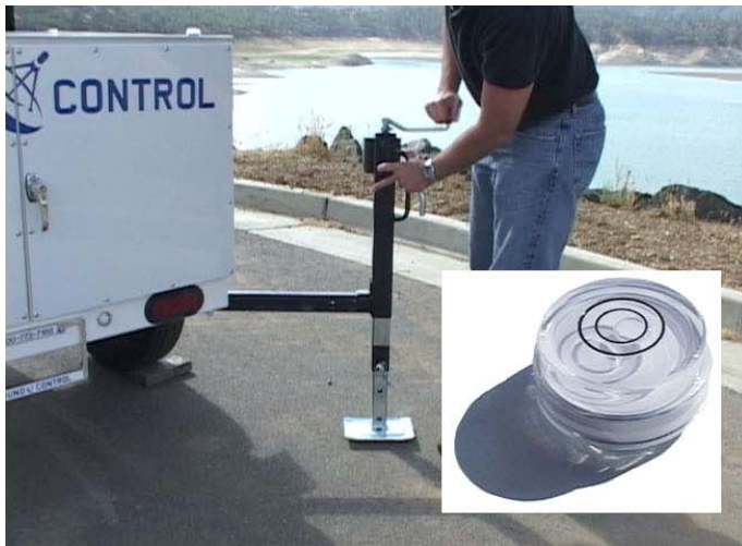
STEP 6 – Crank all jacks to level the trailer.
