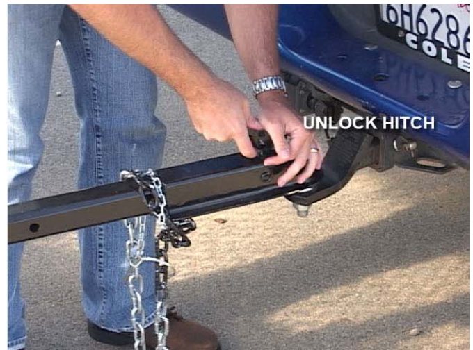
STEP 3 – Pull the pin the holds the front wheel jack against the trailer frame. Rotate it 90 degrees so that the jack locks into place with the wheel side down. Carefully unlock the hitch from the ball.
