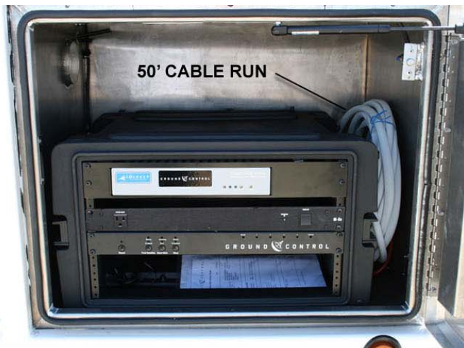
STEP 10 – TURN ON ELECTRONICS. Inside of the electronics case is a portable 6RU rackmount case with an 50 foot cable run that allows you to move the electronics a distance from the trailer. The electronics case includes the iDirect satellite gateway, the 8 AC plug power conditioner, and the Toughsat wireless controller. Both the gateway and controller should power on (lights will appear) with the single toggle switch on the power conditioner.
