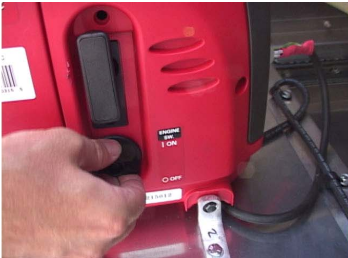
Turn on the POWER Switch to ON, and then firmly and quickly pull the starter cord to start the generator. IMPORTANT - Make sure to turn off the choke after the motor has started.
