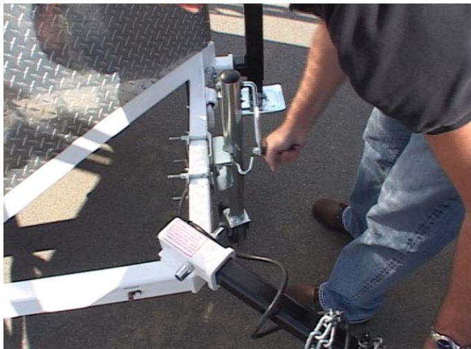
STEP 4 – Begin to crank up the front of the trailer so that the hitch clears the 2" ball on the tow vehicle.
