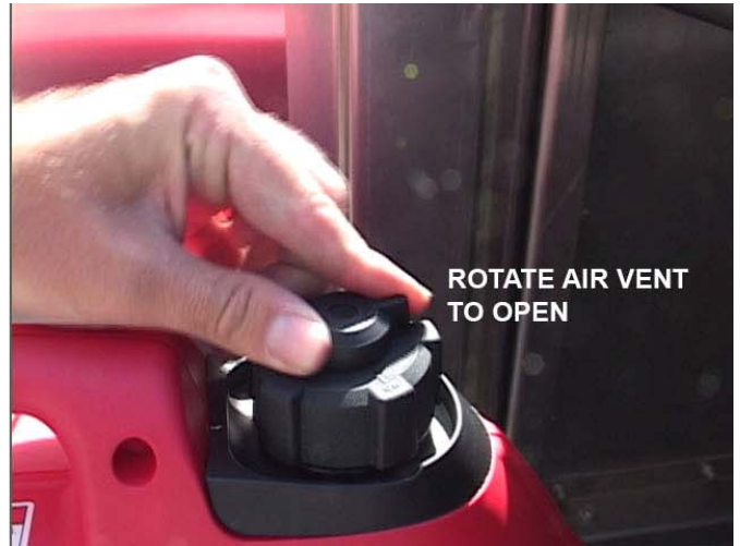
STEP 9. START THE GENERATOR. Close the choke if the generator is cold and open the air vent on the gas cap.
