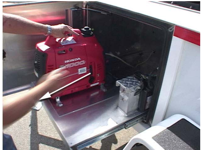
Turn on the POWER Switch to ON, and then firmly and quickly pull the starter cord to start the generator. IMPORTANT - Make sure to turn off the choke after the motor has started.
