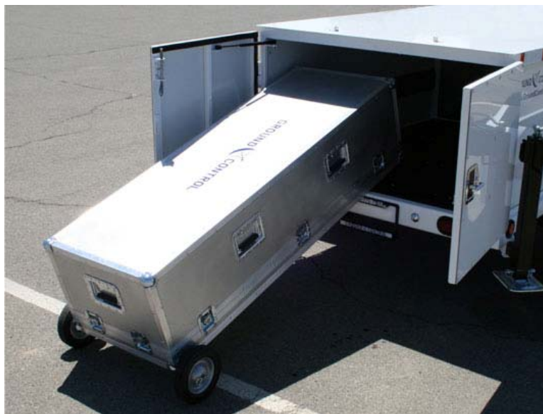
The T-100 trailer can also carry a Toughsat Flyaway case for one-person portability. Use one Toughsat for both systems.
