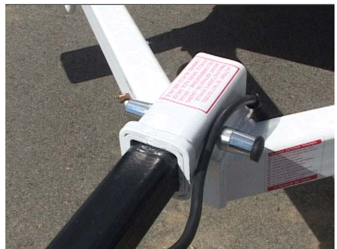
The trailer dolly is a good way of moving the trailer to a different location. Also note the trailer tongue itself may be removed by unlocking the locking pin that holds it to the trailer frame. Removing the tongue may reduce theft of the system, or allow other tongue configurations to quickly be used on the trailer.
