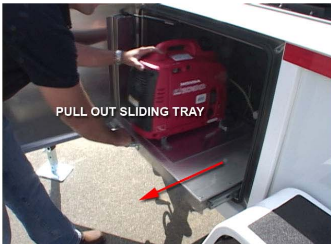
STEP 8 – OPEN THE GENERATOR CABINET, and slide out the generator tray. The hand grip on the tray has a thumb lock to unlatch the rolling tray. NOTE that next to the generator are two toggle switches that turn on cabinet lights or emergency flashers for the trailer. Both are battery operated, and the generator does not need to be running in order to have lights or flashers.
