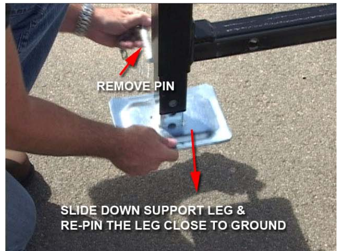
STEP 5 – RETRACT THE SUPPORT LEGS. Although use the supporting leveling legs is not mandatory, it is recommended for high winds or accidental shifting if bumped. Unpin the legs and arms and slide both into place.
