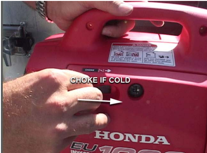
STEP 9. START THE GENERATOR. Close the choke if the generator is cold and open the air vent on the gas cap.
