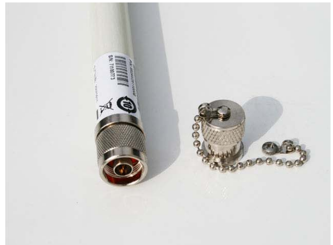
STEP 7 – Hand tighten the two high-gain antennas into the two bulkhead connectors on top of the trailer.
