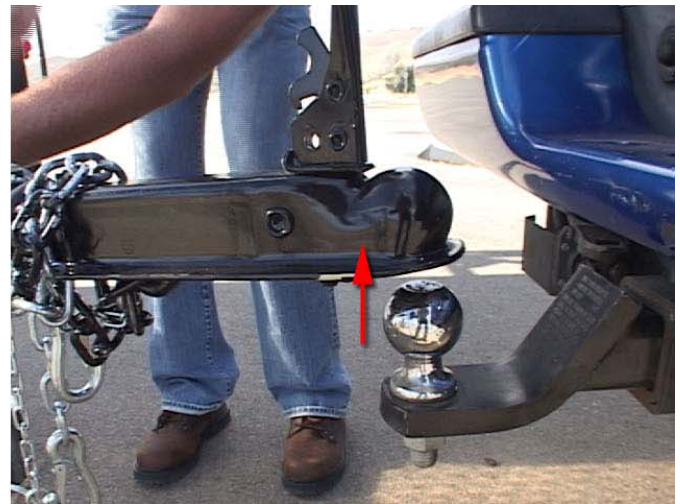
STEP 4 – Begin to crank up the front of the trailer so that the hitch clears the 2" ball on the tow vehicle.
