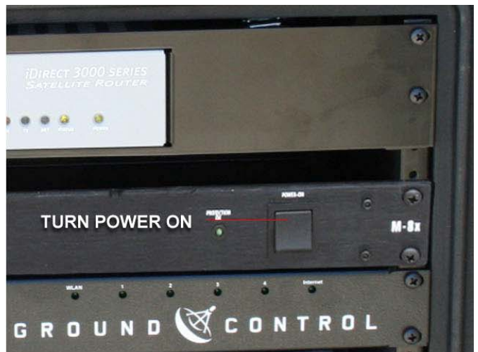
STEP 10 – TURN ON ELECTRONICS. Inside of the electronics case is a portable 6RU rackmount case with an 50 foot cable run that allows you to move the electronics a distance from the trailer. The electronics case includes the iDirect satellite gateway, the 8 AC plug power conditioner, and the Toughsat wireless controller. Both the gateway and controller should power on (lights will appear) with the single toggle switch on the power conditioner.
