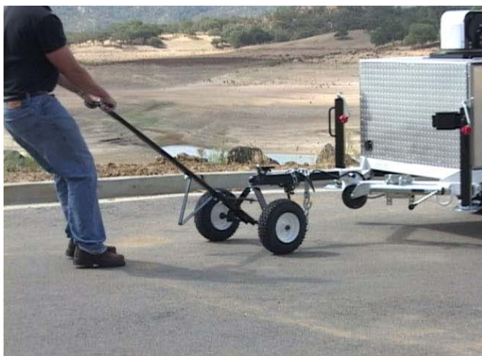
The trailer dolly is a good way of moving the trailer to a different location. Also note the trailer tongue itself may be removed by unlocking the locking pin that holds it to the trailer frame. Removing the tongue may reduce theft of the system, or allow other tongue configurations to quickly be used on the trailer.
