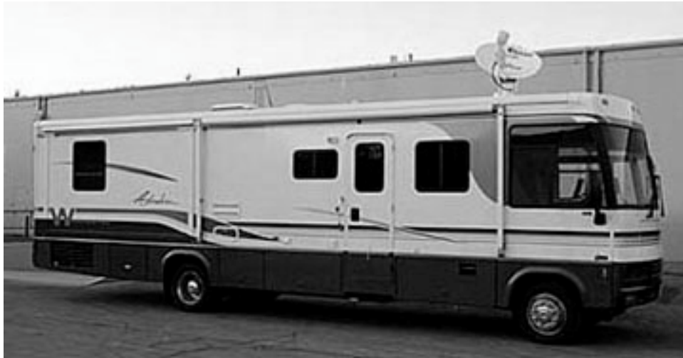
Compliant Installation for Two-Way Temporary-Fixed DIRECWAY Antenna
