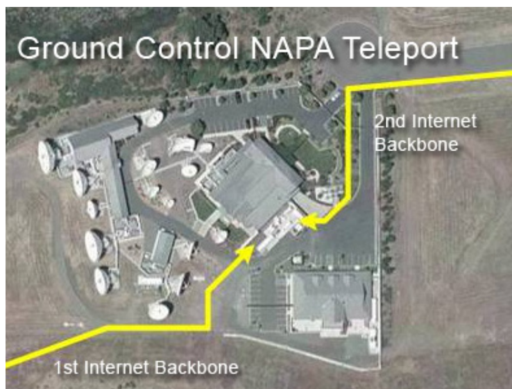
The iDirect Teleport in Napa, California uses redundant connections to the Internet Backbone.
