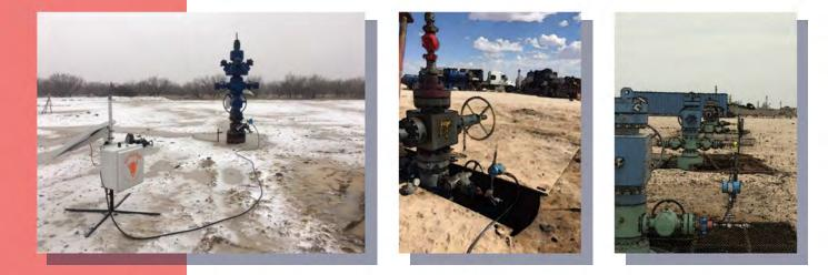
The data requirement for a DFIT is typically one second data resolution and can last days; sometimes weeks. It's completed before the full team arrive on site, therefore, there's no power, and the unit must be powered by a solar array - including the means of transmitting the data back to the engineering team. BGAN devices are known for requiring little power and can run on a 50W solar panel with a 35Ah 12 VDC battery.
