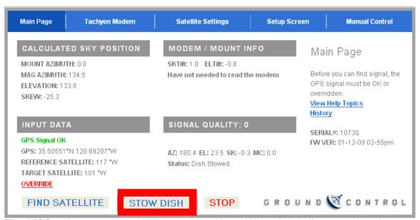
The MSS will now move to its stowed position. When it is fully stowed and ready for travel, the status line will display "System Stowed"
