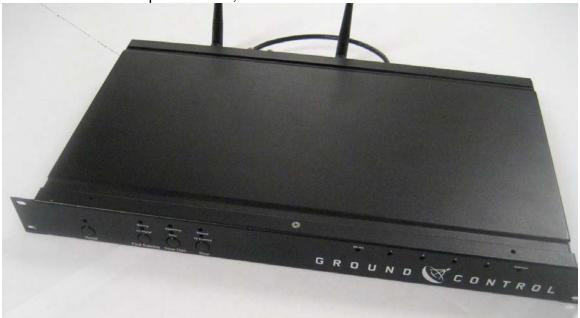
The GC Controller has a power cable and a switch, which need to be plugged in and turned to the "ON" position, signified by the single line.
