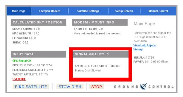
and you will see what the MSS is doing at this moment, in the "Status" line. The MSS will search for signal, and when it's ready, it will display "Passed Test, System Online".
