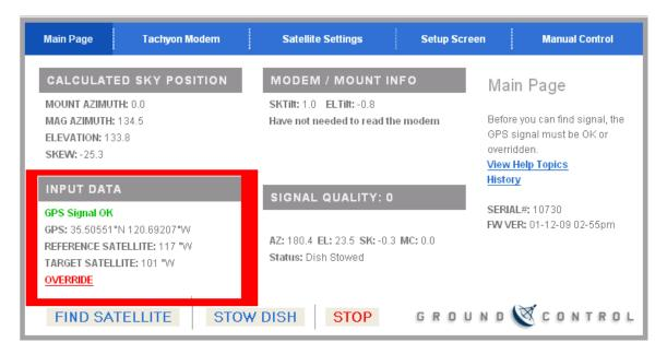
Confirm that it displays "GPS Signal OK" and has GPS coordinates. Without this information, or if the MSS does not display "GPS Signal OK", the MSS will not deploy. Once you have confirmed this, look for "Reference Satellite" and make sure it is the same thing as "Target Satellite". When all of these things are true, click on "Find Satellite"
