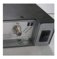
Please note that an iDirect modem does not have a power switch; to power the unit on, simply plug it in.
