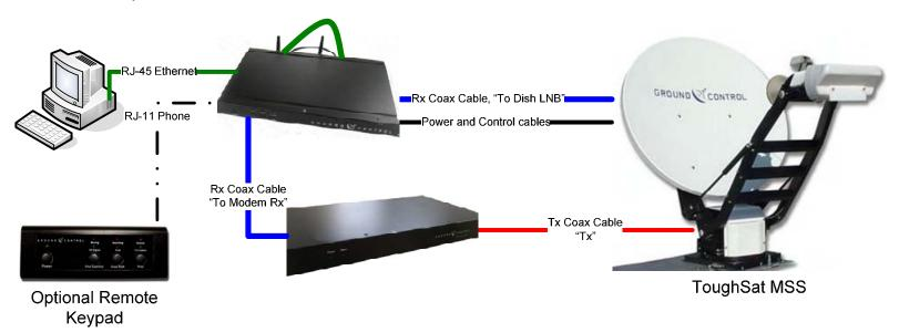
Green lines are standard RJ-45 Cat 5, 5e, or 6 UTP cable. The loop of Ethernet cable on the back of the GC Controller must be connected to both the "Port 1" and "Mount Control" Ethernet ports on the back of the controller.
