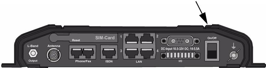
If a switch for the remote on/off function is installed, you may leave the power switch in the “on” position and use the remote switch to turn the terminal on and off. For further information on the remote on/off function, refer to the installation manual for the SAILOR FleetBroadband systems.
