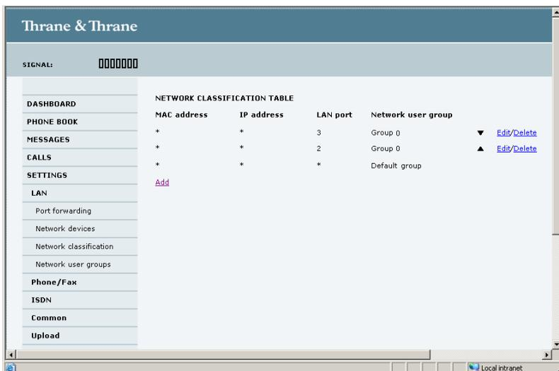
The classification table shows which devices are associated with which LAN ports and user groups. An Asterisk (\*) is a “wild card”, meaning that any value is accepted.
