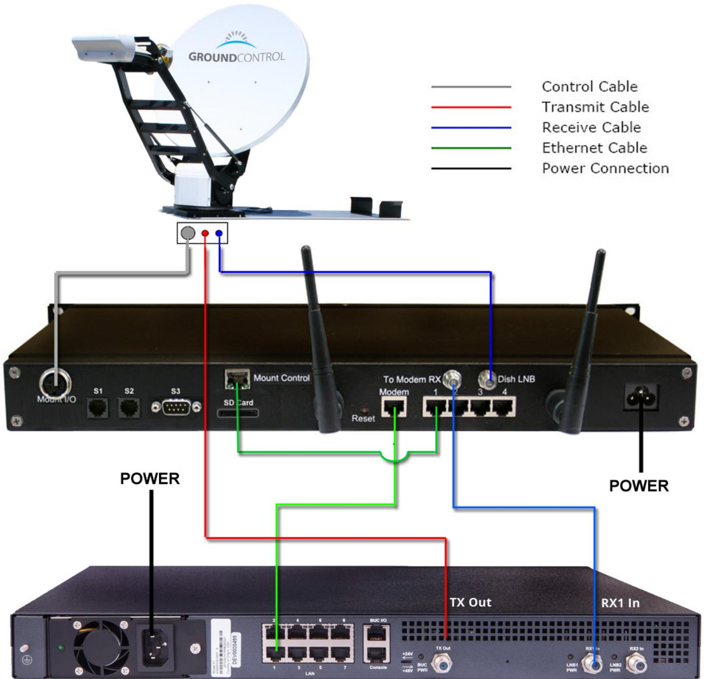
Above is the standard wiring between the Toughsat, the TS2 controller, and the iDirect X7 satellite router.
