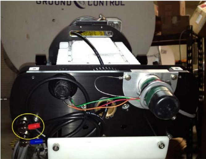
Now you will want to remove the other end of the same cable where it connects to the transmitter, below is an image showing this.
