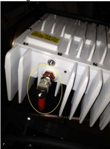
Now connect a new or spare coax cable in place of the one you just removed and power up the unit, after the modem boots up completely (this takes a couple of minutes generally) if this was the bad cable the BUC Power light would illuminate green and your modem would be ready to transmit again.
