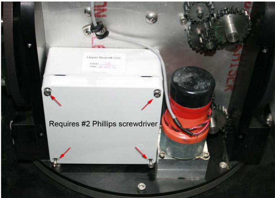
Remove the 4 screws that hold the UCB cover in place.
