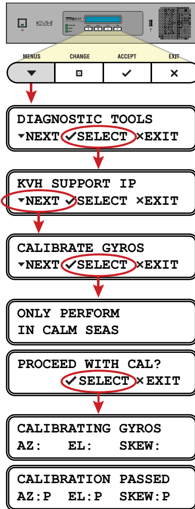
Figure 10-13 Calibrating the Gyros
