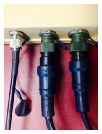
Figure 4-3 Cables Connected: RF, 3-pin and 6-pin respectively
