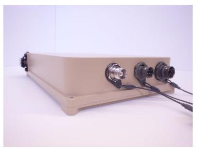
Figure 4-2 Installing Ethernet, Power and RF Cable
