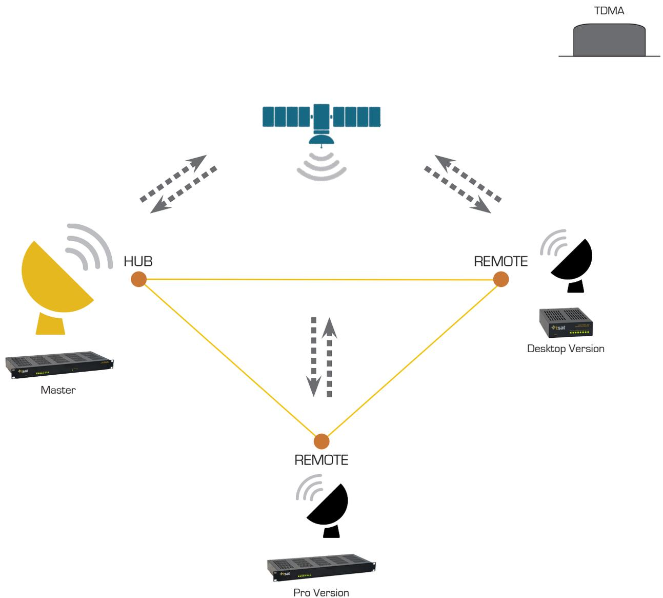
The TSAT 3500 mesh feature (TDD) is implemented with a single TDMA carrier, where the hub is designated as the master. The master provides timing and bandwidth (slot) allocations to the connected remotes in the network.
