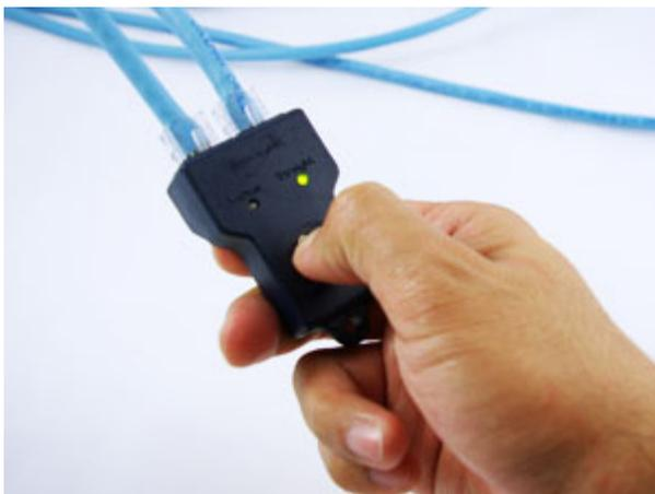
Make sure to test the cables before installing them. An inexpensive Ethernet cable tester does this quite well.
