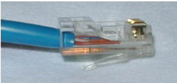
**WRONG WAY** - Note how the cables do not go all the way to the end of the connector.
