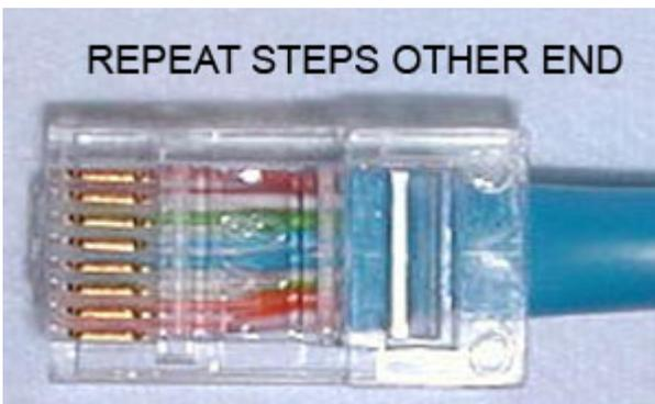
For a standard "Straight Through" cable, repeat all steps and wire color order on the other end of cable. For a cross-over cable, the other end will have a different color order as shown by the crossover picture above.
