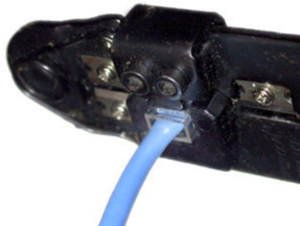
CRIMPING THE CABLE ... carefully place the connector into the Ethernet Crimper and cinch down on the handles tightly. The copper splicing tabs on the connector will pierce into each of the eight wires. There is also a locking tab that holds the blue plastic sleeve in place for a tight compression fit. When you remove the cable from the crimper, that end is ready to use.
