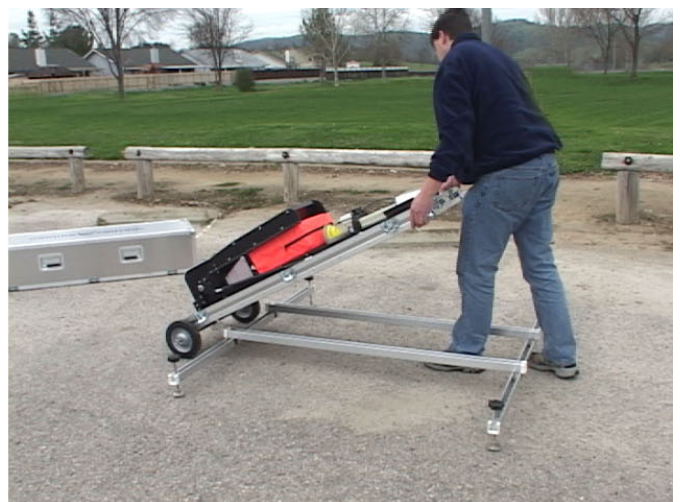
Step 9 – You may now move the bracket to a location where the flyaway will stay. To place the dish on the ground bracket, simply roll it into place.
