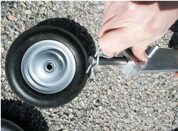
Step 2 – Assemble the dolly. Remove cotter pins from the axle, slide on the wheels, and reinsert the cotter pins.
