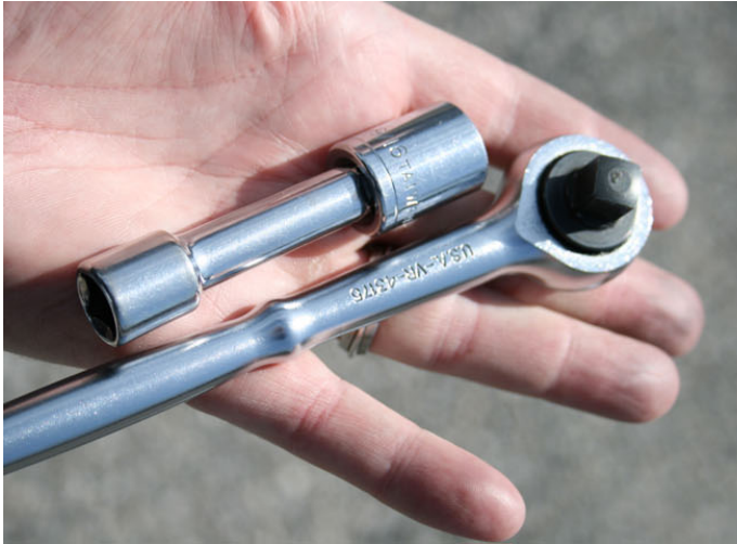
Step 7 - A ratchet wrench and a 9/16 socket is used to secure the four bolts on the rails.
