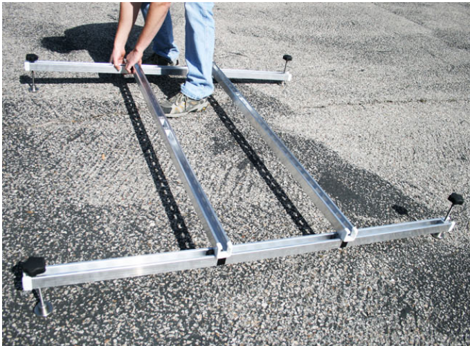
Step 5 – Place the other rails together as shown. Line up the top rails so that ends are above the T-nuts.
