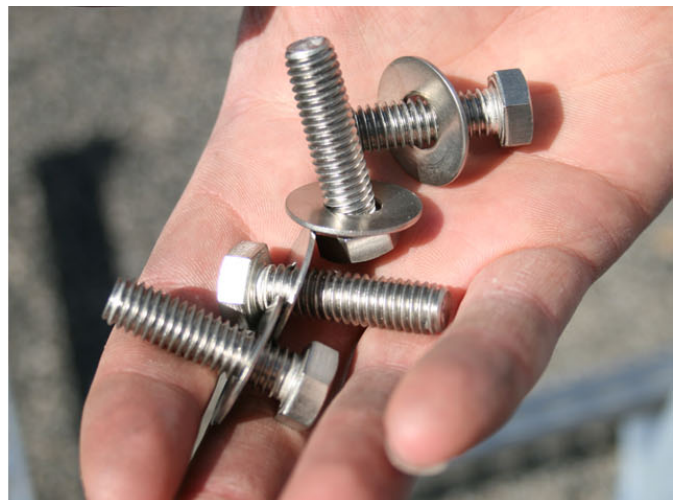
Step 6 - From the hardware pouch, find four 9/16 bolts (with washers) that will secure the rails to each other.
