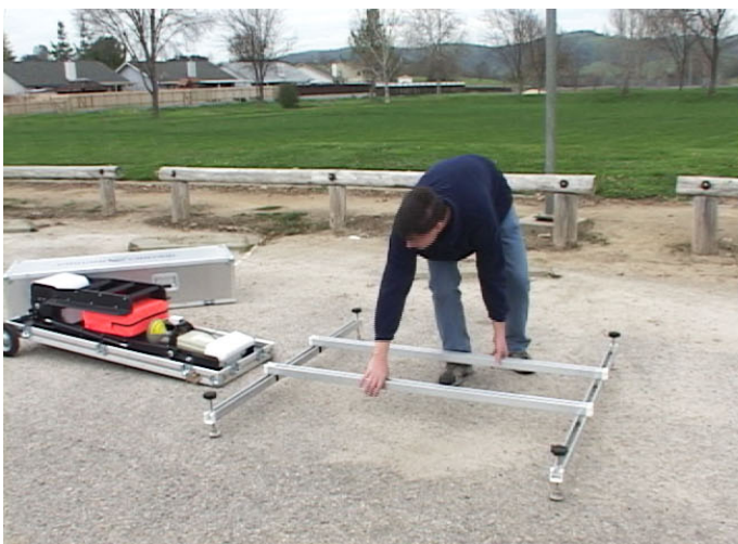
Step 9 – You may now move the bracket to a location where the flyaway will stay. To place the dish on the ground bracket, simply roll it into place.
