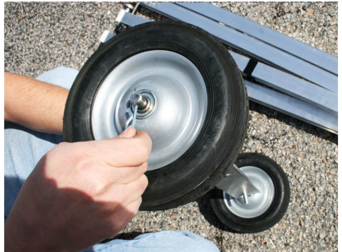
Step 2 – Assemble the dolly. Remove cotter pins from the axle, slide on the wheels, and reinsert the cotter pins.
