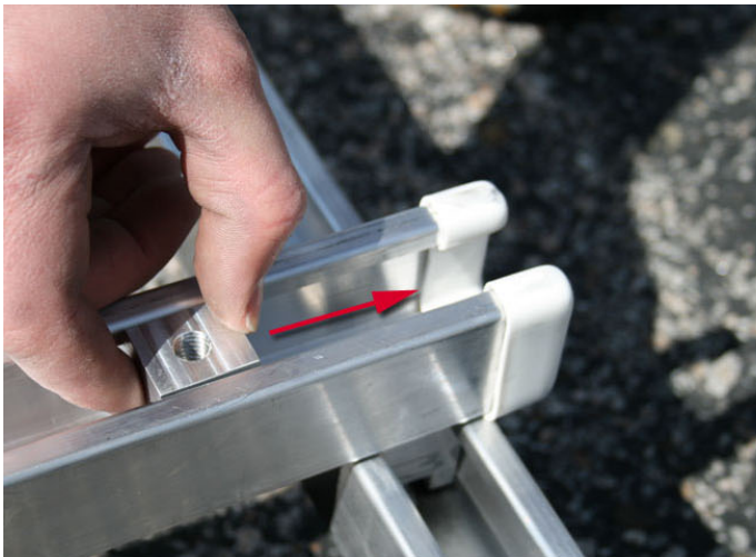
Step 8 – There are four T-nuts on the top rails. Slide them to the ends of the top rails. Note the positions above.
