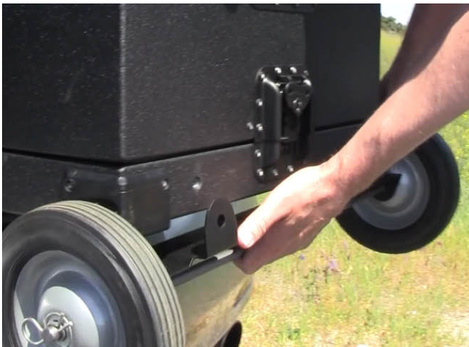
Step 3 – To secure the dolly to the case, slip it into place on the heavy end, and then use the two screw handles to lock the dolly into place.
