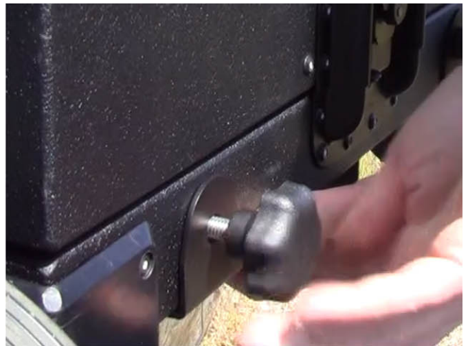
Step 3 – To secure the dolly to the case, slip it into place on the heavy end, and then use the two screw handles to lock the dolly into place.
