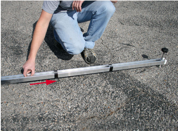
Step 4 – Place one of the rails on the ground and slide the two T-nuts into place on the two black marks.
