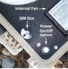
Inside the case is a lighted power button and the SIM card tray. The internal fan helps keep electronics cool if tempretures rise. It is recommended to open the case to help vent excess heat buildup in hot weather.
