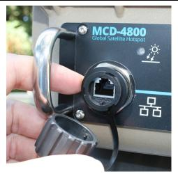
An Ethernet LAN port (RJ-45 with PoE) is available for hardwire connections. When not in use, it is capped to waterproof the case, and waterproof Ethernet connectors are available. Also note the stainless steel bumpers to help protect the front panel from impacts.
