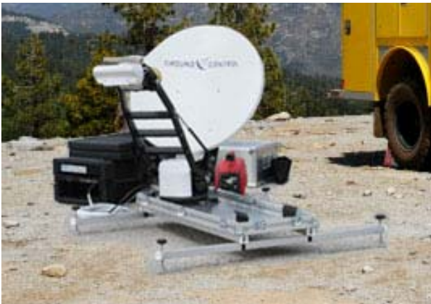
The Flyaway System provides a mobile Hotspot for very high-speed Internet access. More
