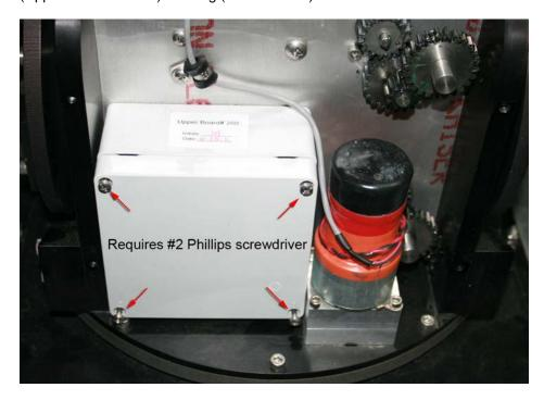
Remove the 4 screws that hold the UCB cover in place.
