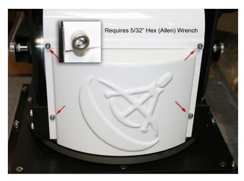
The Toughsat internal parts and electronics are protected by three plastic covers. The front and back covers are held together by the top cover, which must be removed first. After that, the back cover may be removed, exposing the UCB (Upper Control Board) housing (shown below).
