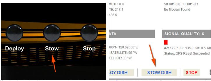
Stowing the dish on the Flyaway can either be done by pressing "Stow" on the Toughsat TS2 panel, or by accessing the controller's web page at <a href="http://192.168.1.2">http://192.168.1.2</a> and pressing on the "Stow Dish" button.
