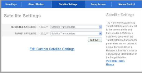
From the drop down menus, select the correct satellite for your system (123W for iDirect). Click "Calculate" You should be able to search again and lock on. If you still cannot lock on, please contact Technical Support.
