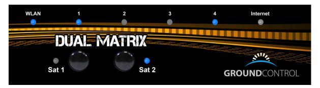
When all of these are active, your equipment is up and ready to search. Connect to the dish control page at 192.168.1.2, then check the input data.
