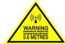
The minimum safety distance is 0.6 m to the side and above the antenna when the EXPLORER 325 is powered. The safety distance of 0.6 m does not apply directly below the antenna, as the radiation forms a hemisphere above the antenna.
