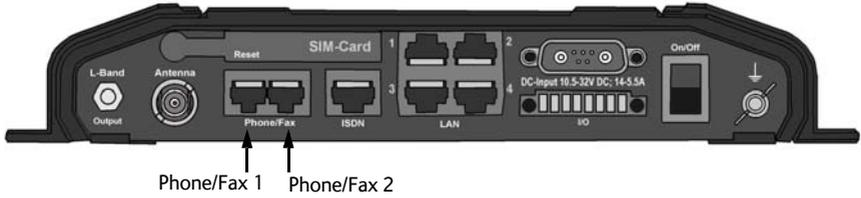
The Phone/Fax connectors are not numbered on the terminal. For configuration, use the numbering indicated on the drawing above.
