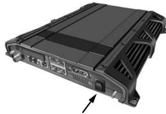
On the 19" rack version of the terminal tip the power switch in the front panel to switch on the terminal.
