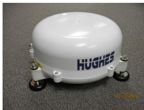
Figure 6-2 C11 antenna unit
