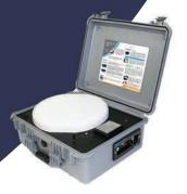
1. PLACE the MCD-MissionLINK case on a flat surface under a wide open sky anywhere in the world. The wider the sky, the more stable the connection since the terminal is connecting with moving satellites.
