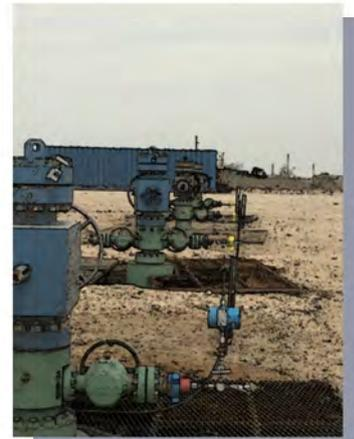
The data requirement for a DFIT is typically one second data resolution and can last days; sometimes weeks. It's completed before the full team arrive on site, therefore, there's no power, and the unit must be powered by a solar array - including the means of transmitting the data back to the engineering team. BGAN devices are known for requiring little power and can run on a 50W solar panel with a 35Ah 12 VDC battery.
