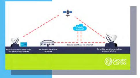
Transmitting your data from your sensors to the satellite, and back to a ground station on Earth, is very secure. What typically happens next is that the ground station sends your data via the internet - protected via a VPN - to your base of operations. This is the most popular choice because it's cost-effective and very secure.
