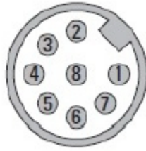
Figure 2-7 Connector Pin Positions
