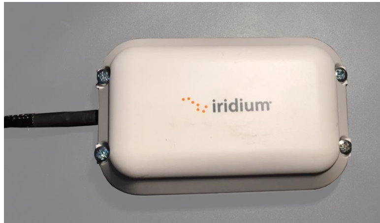
Figure 5-3 Screw Mount Installation
