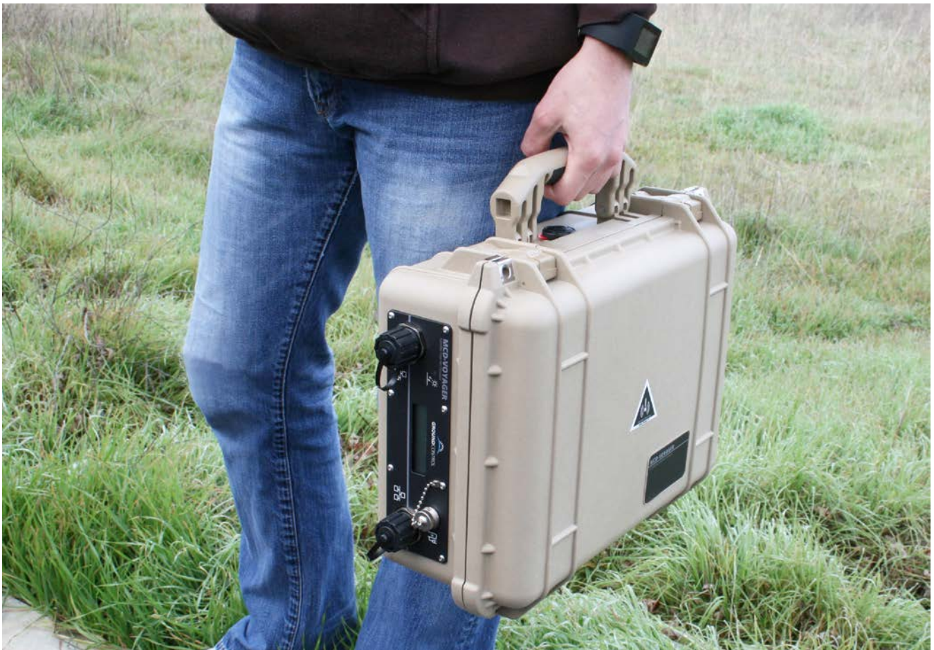
The MCD-VOYAGER is watertight, and operates with the case lid closed.
