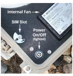
Inside the case is a lighted power button and the SIM card slot. An internal fan helps keep electronics cool when temperatures rise. It is recommended to open the case lid to help vent excess heat buildup in hot weather.
