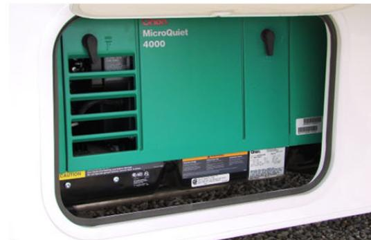
**STEP 2 – POWER OFF** - Check to see that power to the electronics is turned off before starting the generator. This is a good practice to avoid any power spikes or low voltage issues.
