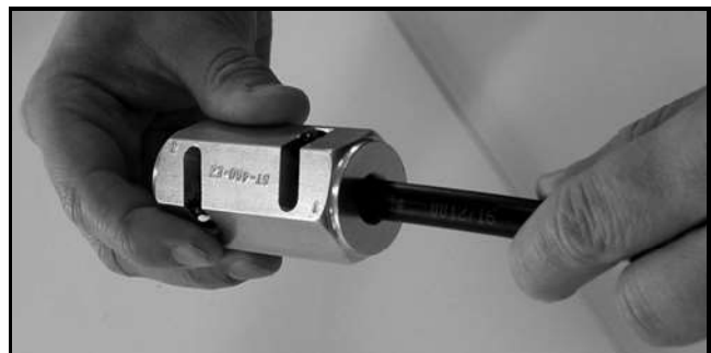
Figure 82: Stripping the End to Expose the Center Conductor
