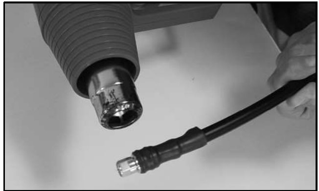
Figure 92: Applying the Heat Shrink Tubing
