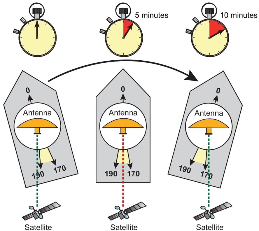
Tracking Avoidance Zone = 170° to 190° (azimuth)
