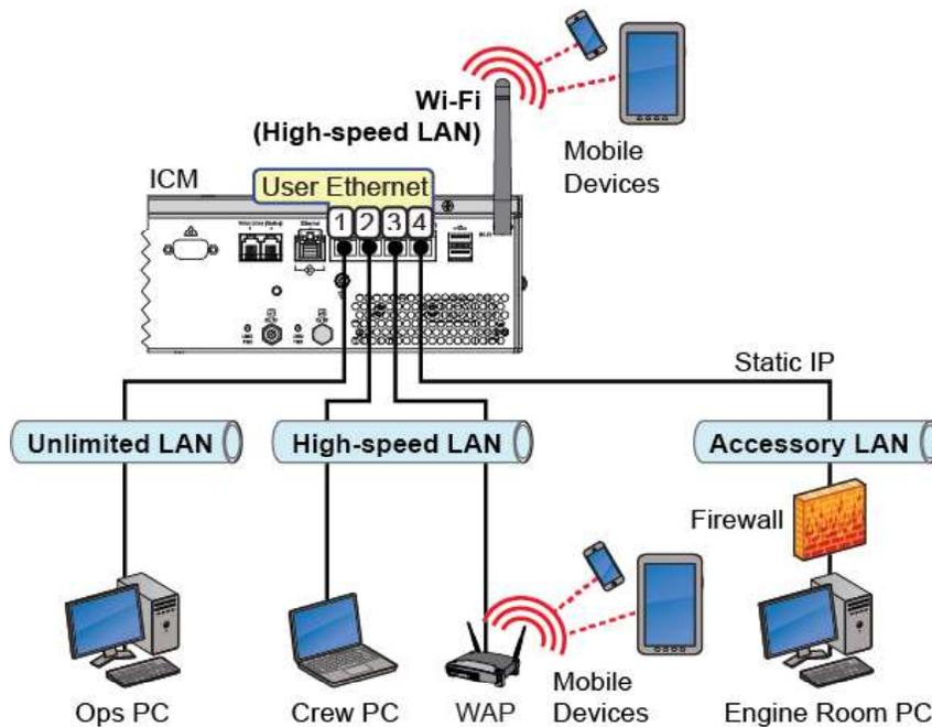
To set up the network in an access control configuration, follow these steps:
