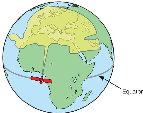
In addition, since satellites are located 22,300 miles (35,900 km) above the equator, the TracPhone antenna must have a clear view of the sky to transmit and receive signals. Anything that stands between the antenna and the satellite can block signals, resulting in lost data.
