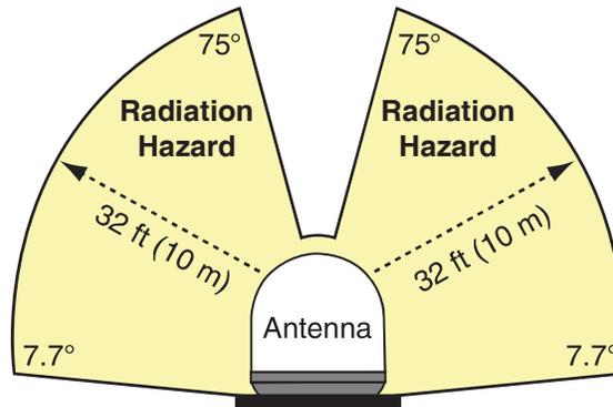
NOTE: You can set up no-transmit zones to inhibit transmissions within areas frequented by passengers and/or crew. See ["Establishing No-Transmit Zones"](#) on page 33 for details.
