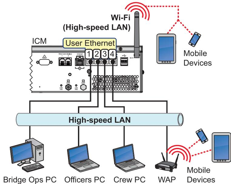
4. Make sure all computers are configured for DHCP addressing (see [“Configuring Computers for DHCP” on page 72](#)). Devices connected to the ICM (via Ethernet cables or Wi-Fi) will receive IP addresses from the ICM via DHCP. The ICM serves as a router.
