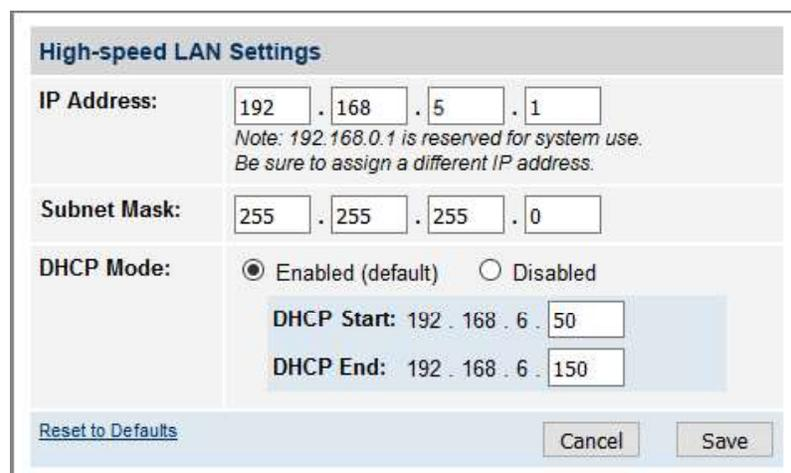
The screenshot shows the 'High-speed LAN Settings' configuration page. It includes fields for IP Address (192.168.5.1), Subnet Mask (255.255.255.0), and DHCP Mode (Enabled (default)). Below the DHCP Mode, there are fields for DHCP Start (192.168.6.50) and DHCP End (192.168.6.150). At the bottom, there are buttons for 'Reset to Defaults', 'Cancel', and 'Save'.
