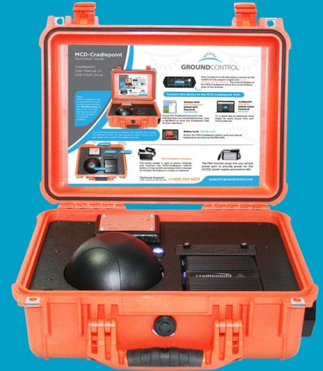
**A Self-Contained 3G/4G/LTE CradlePoint 900** in a carry-portable ruggedized Pelican case that operates for up to 10 hours on the internal battery. Operation is one-button easy and closing the case for all-weather operation. The MCD-Cradlepoint has all the features the COR IBR900 Cradlepoint terminal along with the FirstNet approved MC-400 modem for public safety. This terminal operates in extreme environments for powerful cellular communication for any industry at any time.
