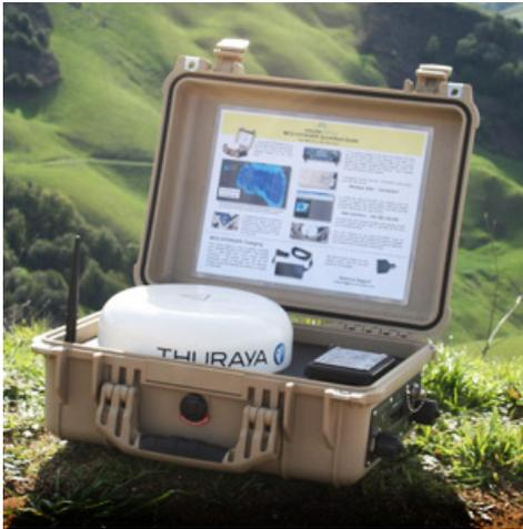
Simply place the MCD-4800 under an open sky, on top of a rock, a moving car, an ocean vessel and turn it on. It connects to the satellite and creates a Wi-Fi hotspot for any in-range laptops or other wireless devices.
