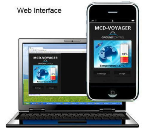
The MCD-Voyager web interface can be accessed by any connected browser. Screens show battery life, data usage, wireless security settings, MAC address filtering, SMS messaging screens, and many other parameters.
