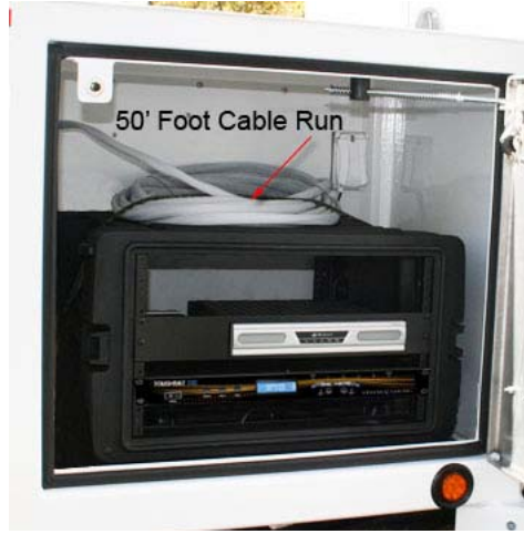
A 6RU rackmount case is locked behind a stainless steel weather-proofed trailer cabinet door. The rackmount case itself can be moved up to 50 feet from the trailer, and placed inside of a structure or tent if desired.
