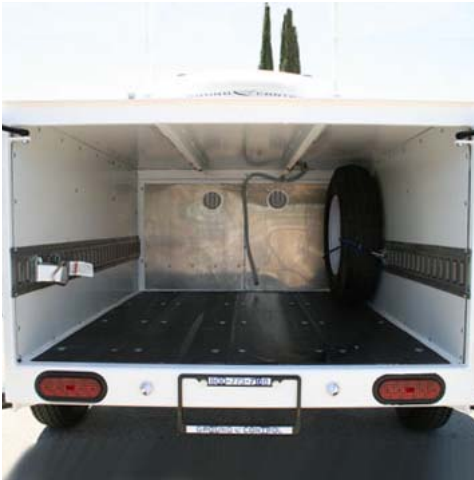
The weather resistant enclosed rear lockable storage bay includes a spare tire. Interior dimensions are 62"L x 46"W x 24"H. Quick lock side straps keep loads secure while moving.
