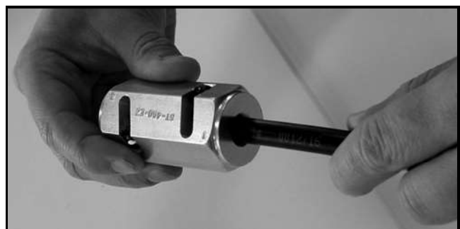
Figure 101: Stripping the End to Expose the Center Conductor
