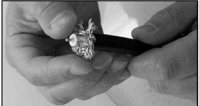
Figure 106: Flaring the Braid
