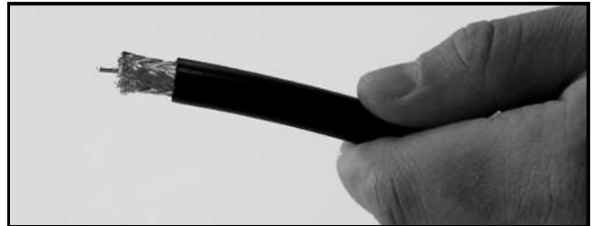
Figure 104: Cable Stripped, Exposing Dielectric
