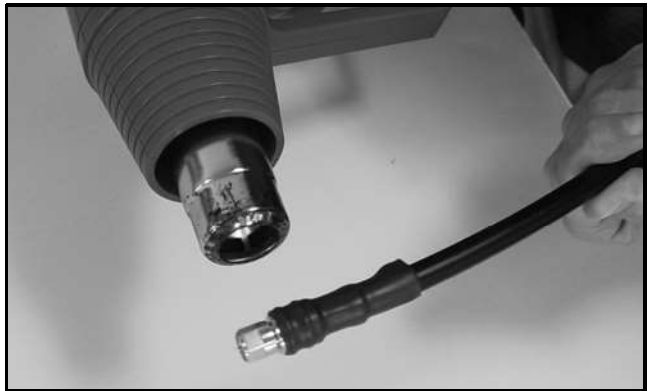
Figure 111: Applying the Heat Shrink Tubing
