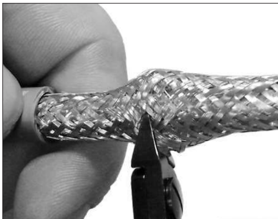
Figure 33: Cutting the Cable Braid Bulge
