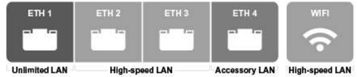
Figure 74: Open Access HTS Configuration
