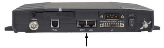
For information on how to connect to the interfaces, see the installation manual for the EXPLORER 325 system.
