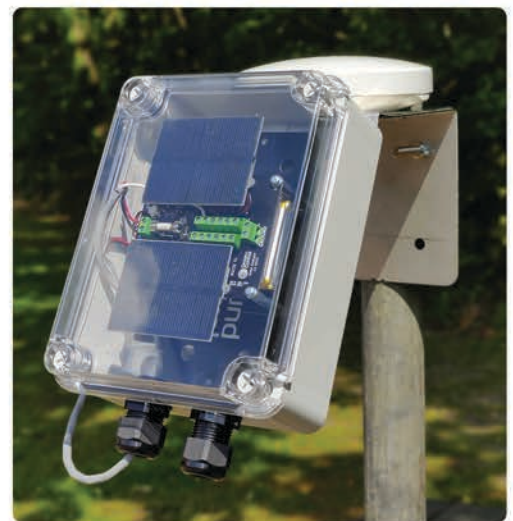
Showing RockBLOCK Sense powered by a combination of Lithium-based cell and supporting solar panel for Arctic location
