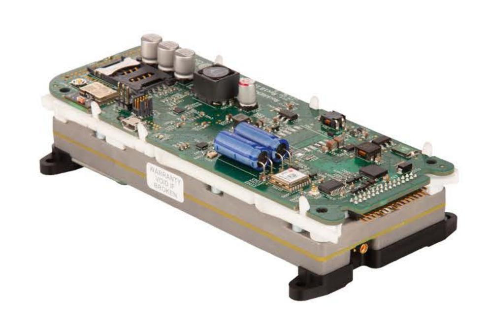
Leveraging the Iridium Certus 100 satellite airtime service, RockREMOTE Mini OEM provides a lightweight subassembly for easy integration into a new product or IoT system. Add a Certus antenna, power and an Ethernet/IO interface, and the kit has everything needed to apply satellite data connectivity to a remote IoT LAN/WAN project.
