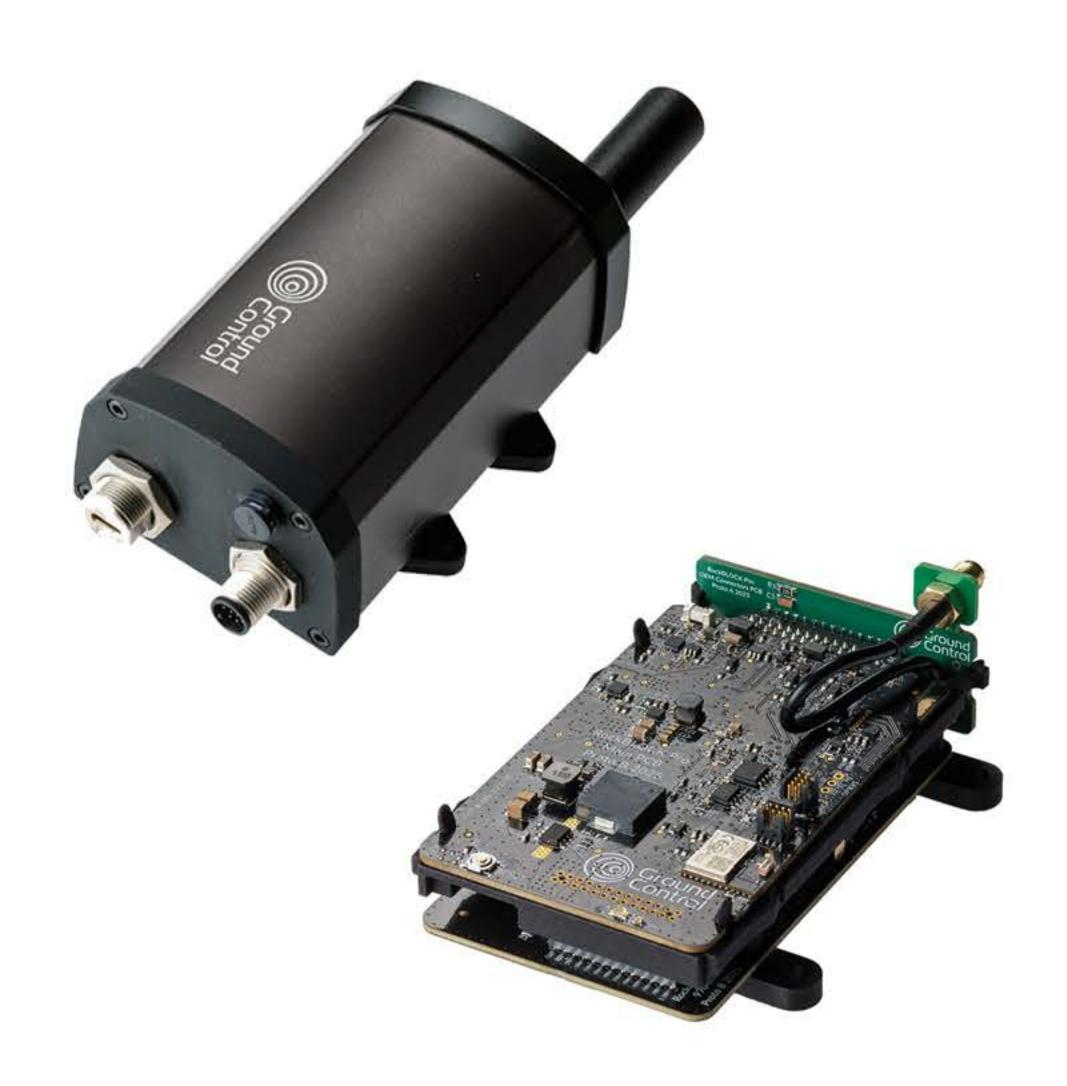
RockBLOCK Pro and Pro OEM: plug and play satellite IoT and tracking terminals powered by Iridium Certus 9704 for faster, larger messages.
