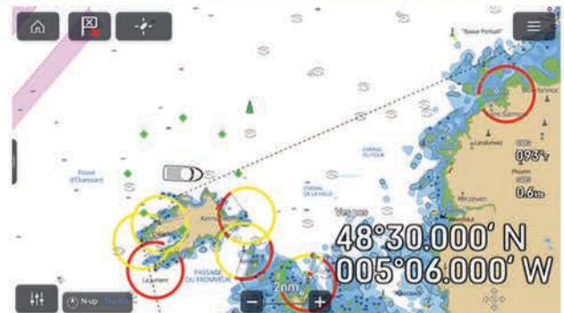
Above: The APNT position (the boat) compared to the GNSS position (the green triangle) which may be spoofed. The circle of green dots indicates the current EPE (Estimated Position Error) of the APNT signal.
